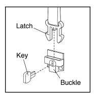
it counterclockwise 1/4 turn. Always keep the buckles locked when the spa is not in use. Keep the keys in a safe place, out of the reach of children.
